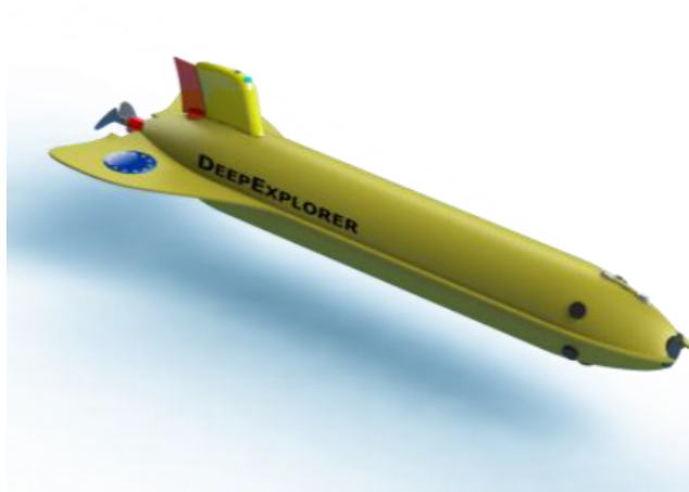
Figure 2.1 - Early Concept for the BRIDGES Deep Explorer Sub-Sea Glider
